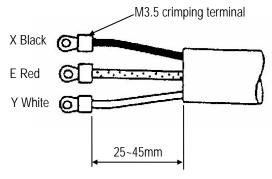
Figure 5.2 Terminal Treatment of Excitation Cable
